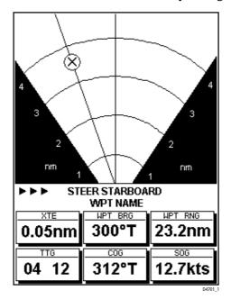
The line to the waypoint symbol is shown at an angle equal to the difference between the COG and the Bearing to Waypoint. The waypoint symbol is the symbol of the target waypoint as seen on the chart.
